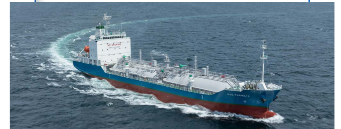
PGC PERIKLIS Fully-Pressurized Gas Carrier SIZE: 7,500 cbm Built in: 2017
